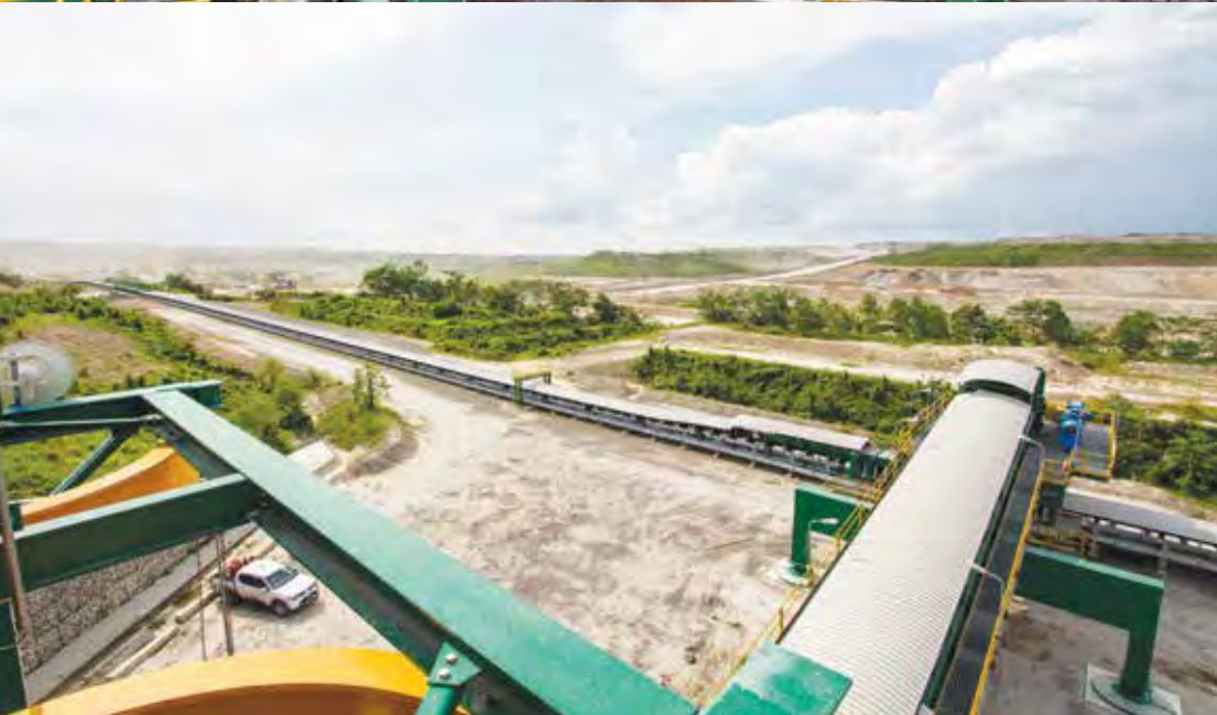
In 2013, construction was completed and trials began of the new out-of-pit overburden crusher and conveyor system at Al's Tutupan pit. Left, coal is delivered to the crusher and fed into the 10km-long conveyor. Right, at the end of the conveyor a computer-controlled arm on caterpillar tracks disposes of the crushed rock by spreading it in thin layers.
