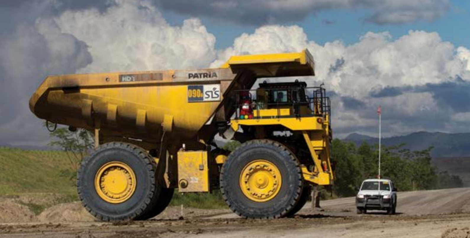
The movement of traffic inside our mining areas is strictly controlled and safety is paramount to minimize accident risks. Heavy dump trucks have priority and regular vehicles always carry high pennants to aid visibility for the truck drivers.
