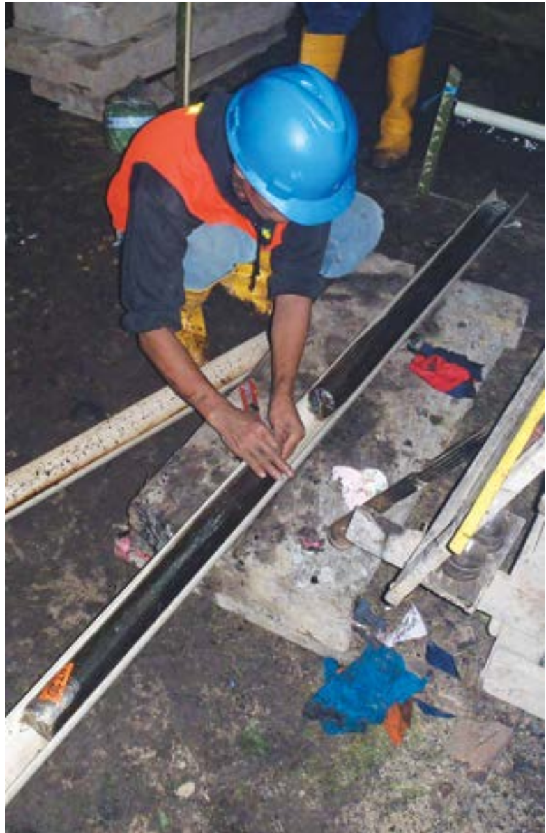
A site geologist gives a coal core sample from BEP a protective plastic wrapping before taking samples. BEP’s coal is low-rank at around 3,350 Kcal/kg.
