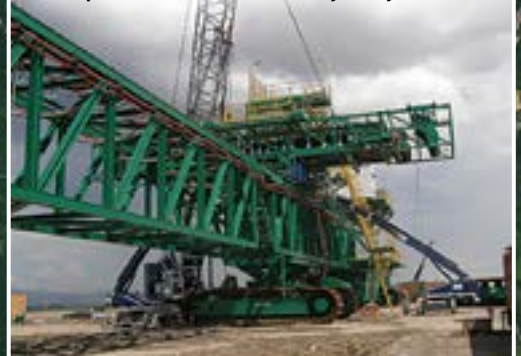
The spreader makes arcs on giant tracks and spreads overburden evenly in layers.
