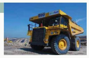
Komatsu mining dump truck operated by Bio Diesel Fuel (BDF)
